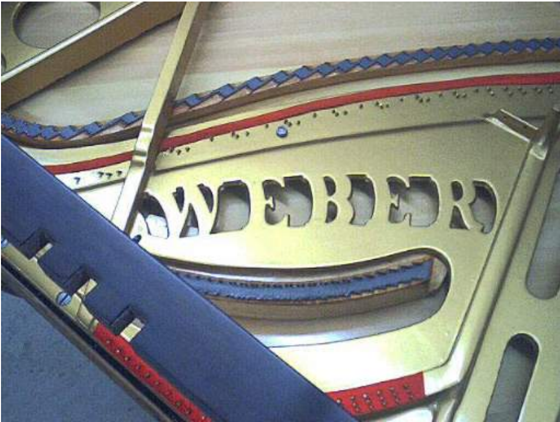
The Weber name is cast into the plate as part of the freeze-out holes. Something that on an upright probably only a technician would ever see.
