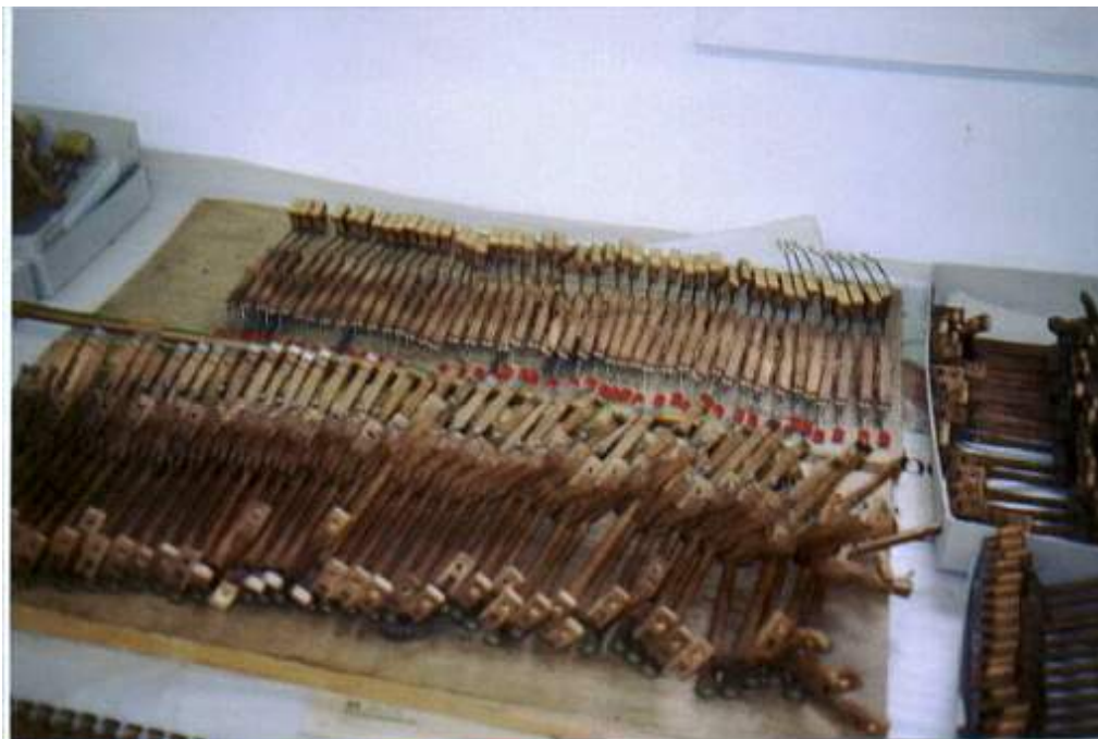
Notice sostenuto tabs on damper levers. Each action part was removed and individually shell blasted for cleaning and then rebuilt as necessary. Parts on right before shell blasting.
