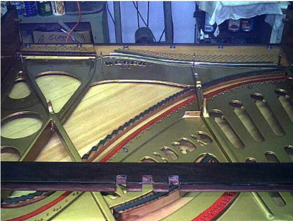
This photo shows the new soundboard and notice the open face pinblock. The piano was original 1/0 tuning pins and is being restrung with 2/0 pins
