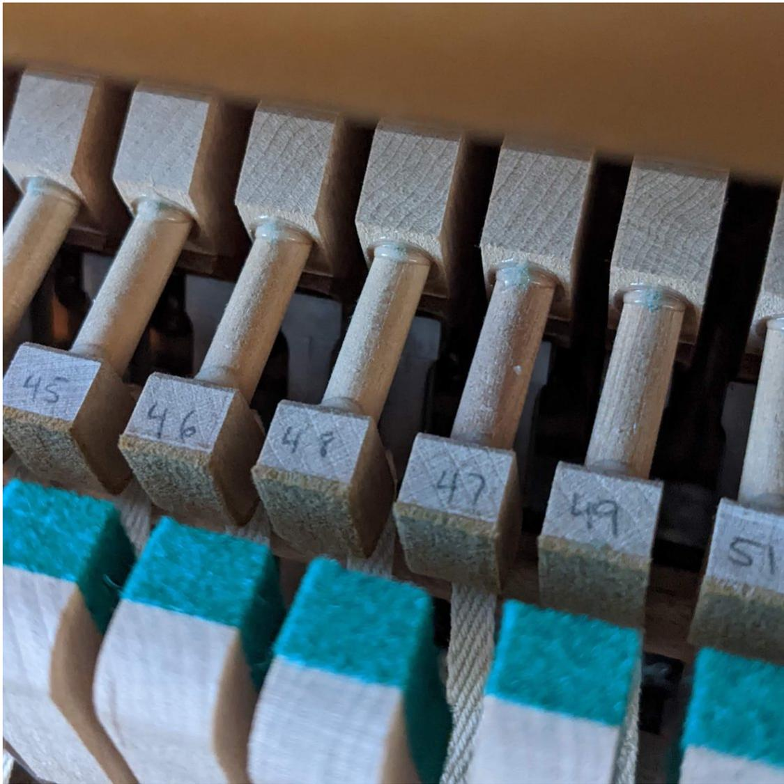
*A numbering mistake, or a reinstallation mistake? This was on a Yamaha P2 which had its hammer return spring threads replaced years ago: with grooves thoroughly formed, I let this one slide. - Andrew Kovaleski*
