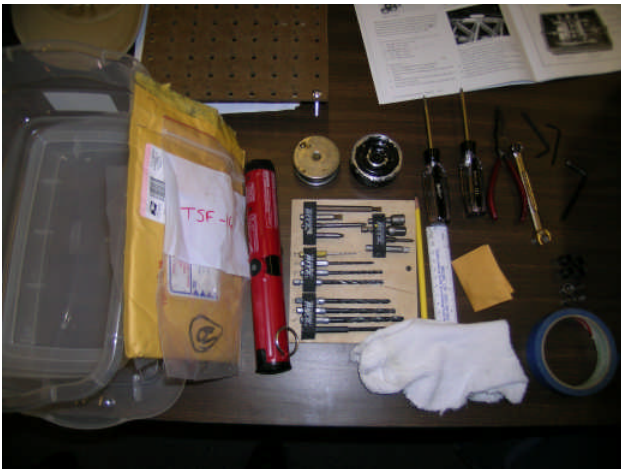
Basic tools required for the job include electric screw driver and #1 & #2 phillips head, hex wrenches, masking tape, replacement bushings, and hex head screws, some cleaning materials.
