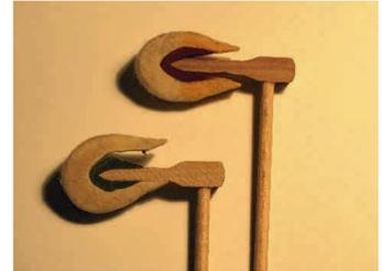
With the hammer clamped and secure use a Dremmel tool with drill no. 69 to drill two holes through the hammer felt and wood.
