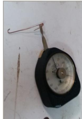
Bryan Hartzler showed us how he was measuring and modifying the spring tension on damper underlevers in a back action. He recently bought a spring gauge and was measuring the tension in some of the springs, some of which were more than double what some of the factory specs may have called for.
