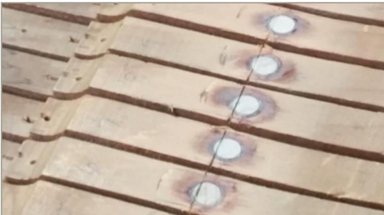
showing where the center of the capstan line is and he used a marking guage, or sharp edged tool, to mark that spot on the key. A pencil line may be too thick and it is better to lightly etch the mark for better accuracy.
