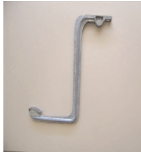
The rocker lift arm. Note the “hump” at the top of the arm between the screws to lever the arm.
