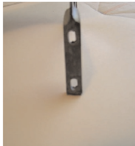
Two screws attached rocker lift arm to the key and would be levered to adjust for lost motion.
