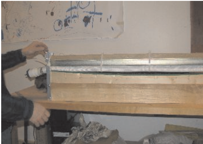
Bryan has a very complete workshop, including a set of soundboard clamps/cauls which utilise a pressurized fire hose.
