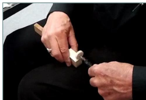
After this, Larry buffed the key using a dremel tool with a buffing wheel and some white buffing compound. Remove tape as needed. Also, keep the buffer moving without staying in any single spot for very long. Otherwise the surface may heat up and compromise the repair.
