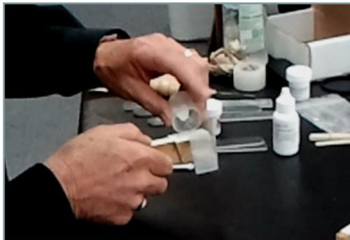
Using a mixing stick or toothpick, apply mix to the key. It may be runny at first, so use the stick to manipulate the mix as needed to coax it into place as it coagulates. Holding the repair end upward may also help. Generally, the puddy will harden within minutes. It is advisable to build up the material slightly higher than the actual key surface, then sand it back down to match later.
